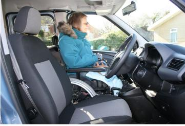
LOWERED FLOOR PROVIDES EXCELLENT EYE-LINE HEIGHT FOR UPFRONT PASSENGER
