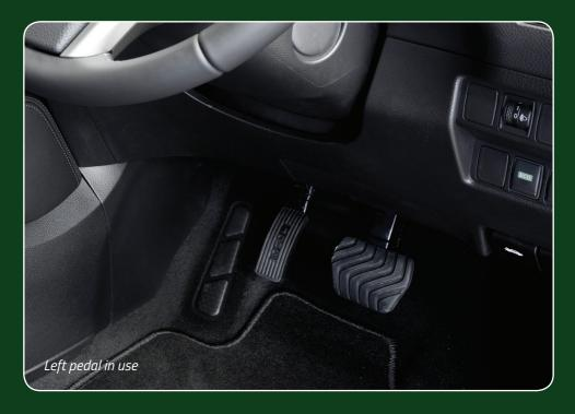
The twin folding left foot accelerator is suitable for automatic vehicles with a pedal which hangs down from the bulkhead. For vehicles with a fully electric floor mounted pedal, please refer to our electric left foot accelerator leaflet.
