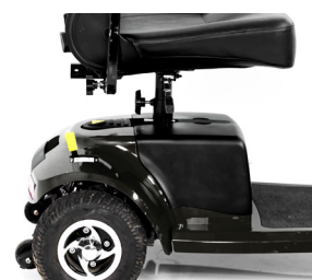
Lithium Vantage Battery Box weighs 6kg
