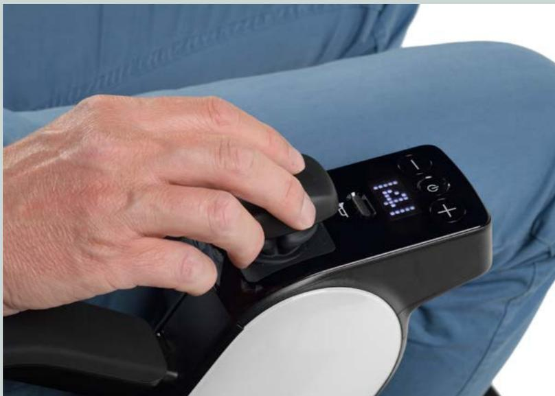
Comfortable controls for effortless steering and safe manoeuvrability including four speed settings, a safety horn and battery life indicator.
