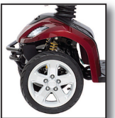
Front oil dampened suspension
