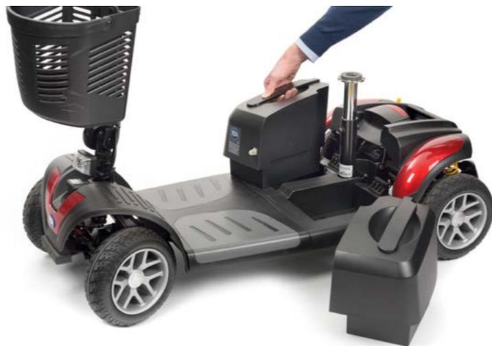
Split twin batteries for easier lifting
