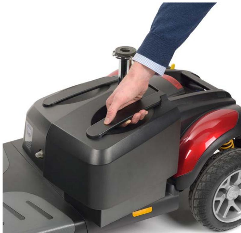
Simple release mechanism for removing battery packs
