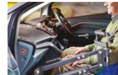
Electric person hoist
